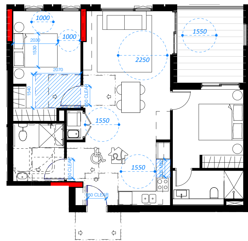
5 POST-ADAPTABLE 2B LAYOUT (2B-02) 1 : 100
